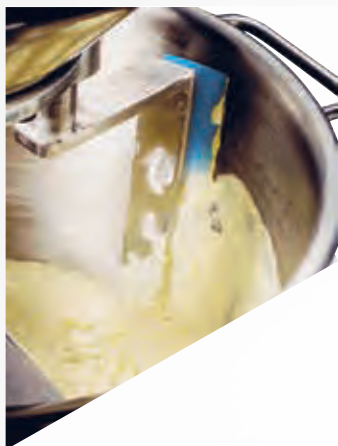
Patented scraper for homogeneous mixing of the ingredients
