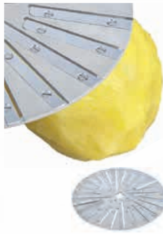
Knife peeling disc smooth surface, peeled hand quality, more waste, hardly any browning, shorter peeling time.
