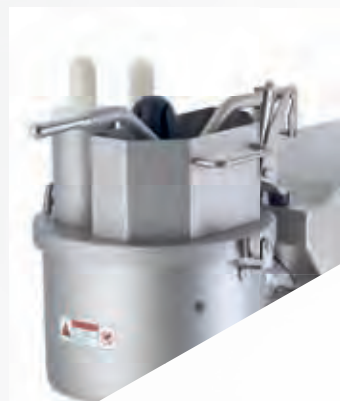
Cutting hopper with double safety switch off
