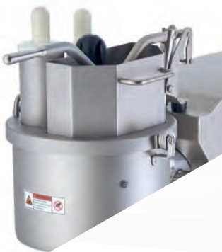
Cutting hopper with double safety switch off
