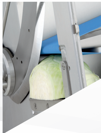
Gentle-touch cutting device ensures precise for clean cuts
